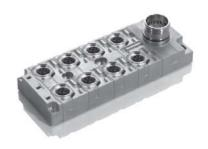
We offer a wide variety of passive actuator/sensor boxes. These allow the user to collect signals in the field and pass them centrally to a controller or to pass signals from the controller to the actuators,
